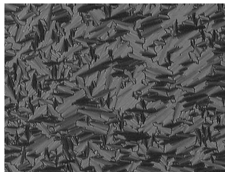
Figure 2. Polarizing optical micrograph of 6:TNF complex on cooling at a rate of 10 \text{ K min}^{-1} .
